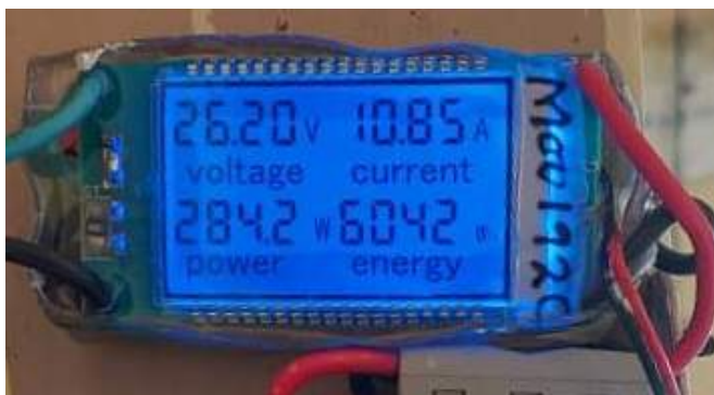
Figure E.1: A PZEM-031 meter that has been encased in clear epoxy resin in Malawi. The energy measurement is in Wh. After 9999Wh, the units switch to kWh.
