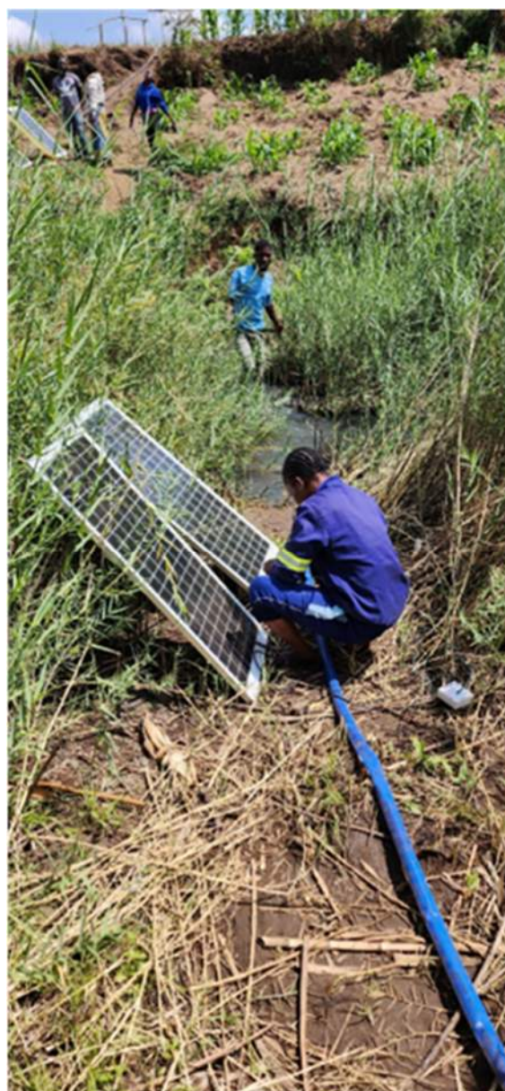
Figure 1: Solar Irrigation Pump System. The solar panels and water-filled lay-flat hose are visible. The pump is submerged in the stream beyond.
