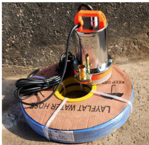
Figure 4: The Original "Small Pump" System. A brushed pump & lay-flat hose are shown. The two 100W solar panels are not shown.
