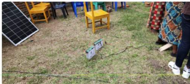
Testing Gilbert's repaired pump in the test pond, using two 18V Forever Batteries in series to simulate full sun on this cloudy day.
